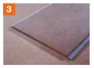
Place glued boards together, bearing in mind that when constructing circular forms the interior radius is smaller than that of the outer board and therefore the two boards are to be of different width.
