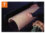
Level both longitudinal edges on the planing machine in order to achieve well-fitting gluing of the upper and lower 'shell halves'. Use locating dowels or Lamello tongues.
