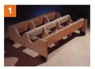
Construct a template out of particleboard. To achieve an exact moulding over the whole surface, keep a maximum distance of 250mm between the ribs.
