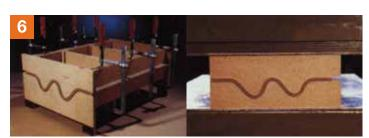
Press the boards together – either by using a screw press or hydraulic press.
