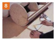
When bonding two halves use gap-filling two-component glue such as Epoxy.
