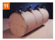
Produce the necessary pressure using clamps. Use sealing tape in the area of the glue joint to prevent the clamps sticking.
